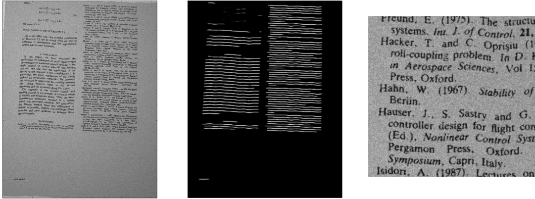
Fig. 5. Text line finding and text/image/math discrimination applied directly to warped, noisy grayscale images. From left to right: (a) grayscale page image with simulated projective transformation, non-linear page warping, an illumination model, and noise, (b) text lines found by the deep text line segmenter, (c) detail from the input page. In addition to text lines being detected correctly, text/math (and text/image, text/graphics discrimination; not shown) also continue to work when operating directly on grayscale images.
