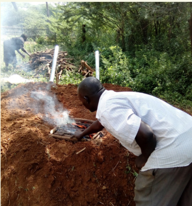
Plate 6. Sealing the lighting point
