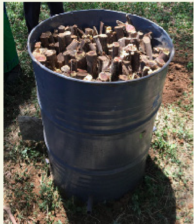
Plate 12. Wood stacked in a DK
