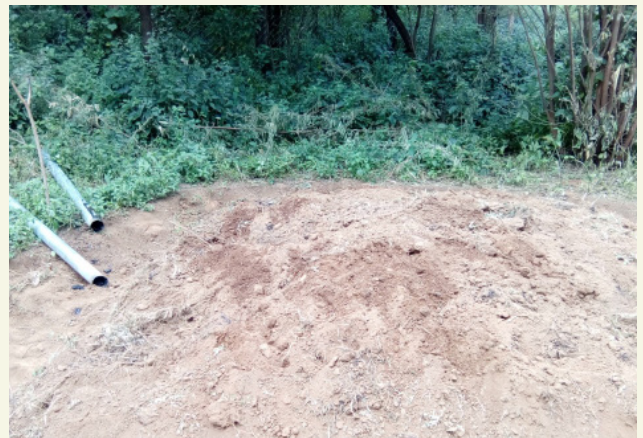
Plate 7. A cooling kiln with breathers and chimneys removed.
