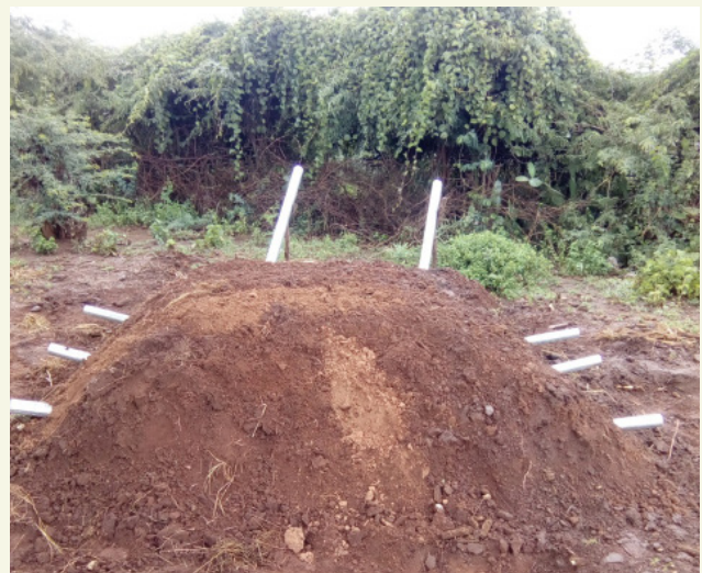
Plate 5. Improved earth mound kiln with two chimneys and six breathers in place, covered with a thick layer of soil (Bourne et al. 2020) Photo by Moses Kirimi/ICRAF, 2019
