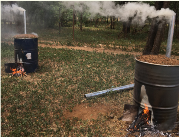
Plate 10. DK without elongated chimney is suitable for charcoal production only.
