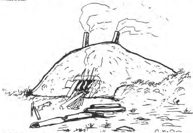
Figure 2.7: Once lit, the kiln emits smoke from the chimneys
