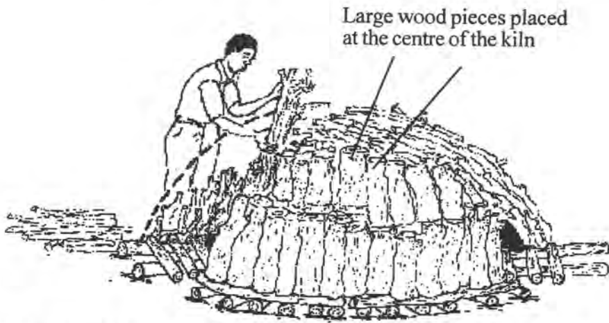
Figure 5.2: Stack wood pieces closely starting with the large pieces of wood at the centre of the kiln and the medium and small-sized pieces around.
