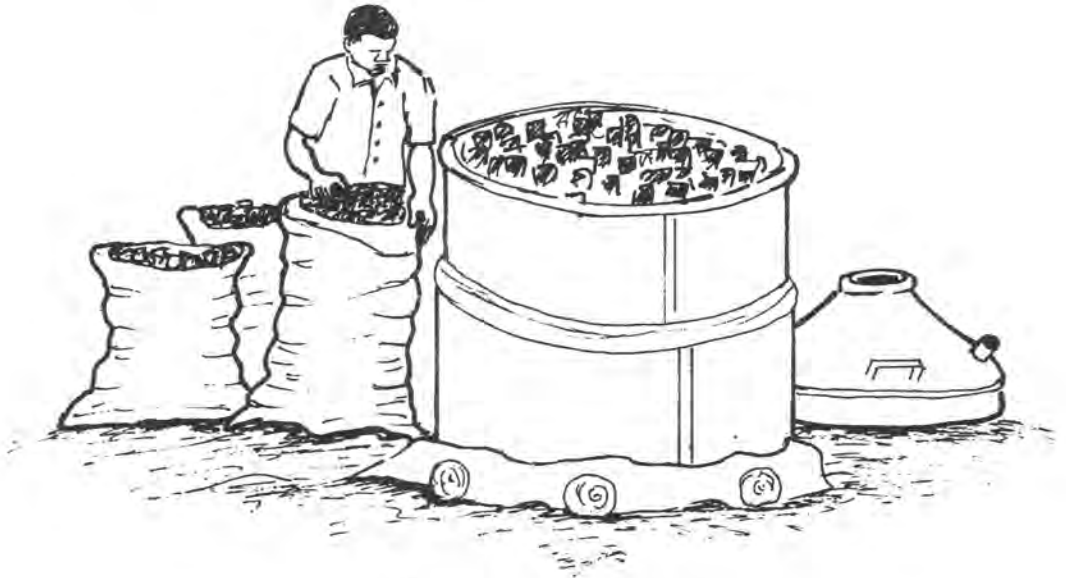
Figure 3.7: The charcoal is removed from the kiln and put into bags
