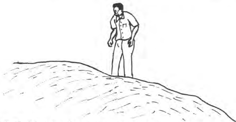
Figure 2.9: The kiln is put off by stepping on top of the earth mound and sealing the chimneys and all other vents to keep the kiln air-tight
