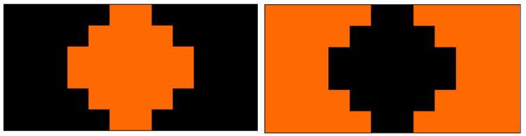
The images above illustrate the display states during a Meatball Flag condition, indicating a mechanical condition or otherwise deemed unsafe to continue. While under the Meatball Flag, the screen will alternate between the two display states.
