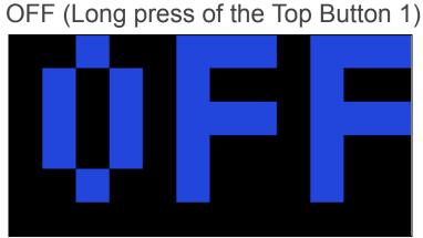
When the device is turned OFF with a long press of the top Button 1, the LED Screen will display OFF for a few seconds.
