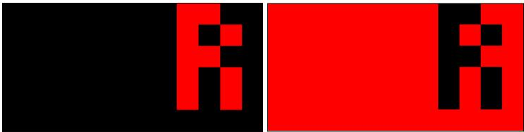
The images above illustrate the display states that occur during a Full Course Red Flag condition. For the initial 10 seconds, the LED Screen will alternate between these two display states. After 30 seconds, the display will stabilize to show the image shown on the right, a majority red screen.
