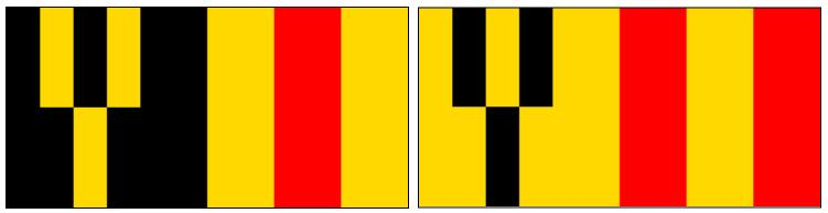
The images above illustrate a dual display state during a Local Yellow Flag condition and a Debris Flag condition, both of which are local alerts controlled by the flag stand. This indicates issues related to both conditions in your current track sector. When this condition occurs, the screen will alternate between the two display states.
