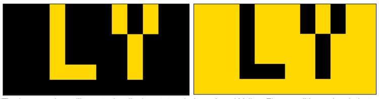
The images above illustrate the display states during a Local Yellow Flag condition, a local alert controlled by the flag stand. This indicates an issue in your current sector. When the Local Yellow Flag is active, the screen will alternate between the two display states.
