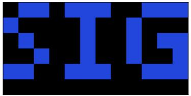
When the device is turned ON in an area without an active Flagtronics network, the LED Screen will display SIG representing that it is not receiving a signal.
