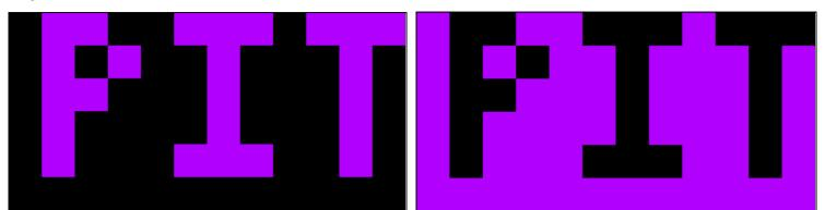
The images above illustrate the display states during a PIT Flag condition, indicating that race control is trying to bring you into the pits. While under the PIT Flag, the screen will alternate between the two display states. This is often provided as a courtesy if race radios have failed.
