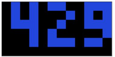
By pressing and holding both Button 1 and Button 2 simultaneously, the LED Screen will display the last 3 digits of the device serial number.
