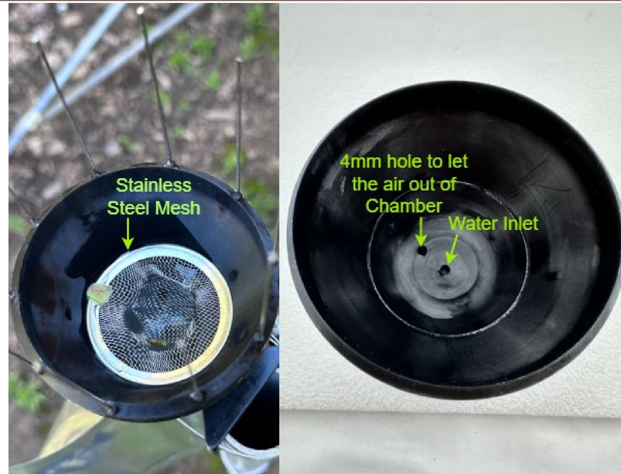
Figure 3. The top part of the Isotopic Sampler is funnel with 80mm of diameter and inside the funnel is a stainless-steel mesh to prevent blockage. The funnel is screwed to the chamber and directs the water to chamber through 4mm hole at center and let the air out through 4 mm hole at the edge.
