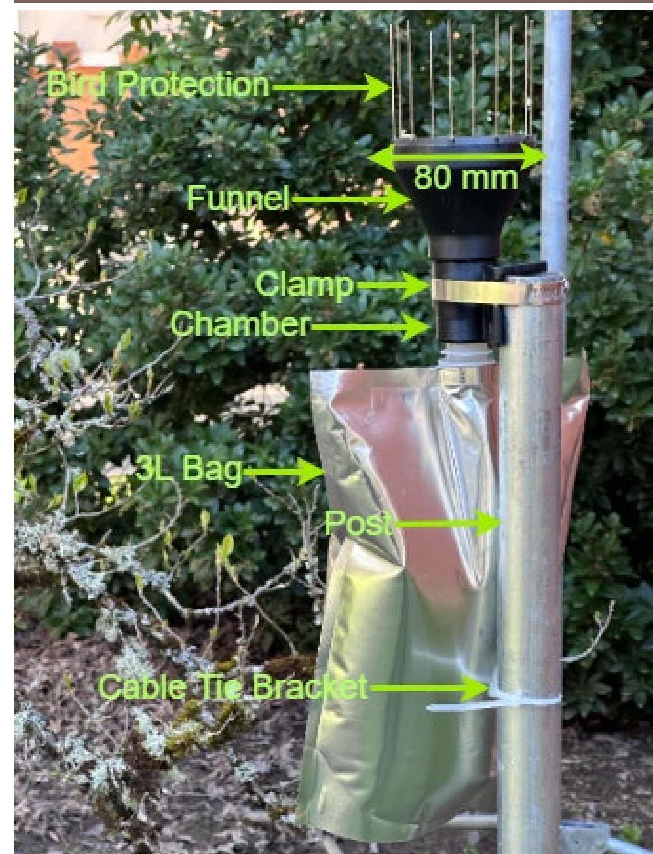
Figure 2. Isotopic Sampler deployed in strength test (full 3 l)
