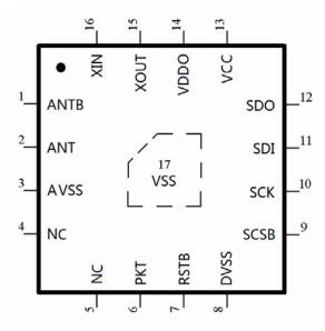
Note: MODE pin is connected to VSS in the chip, so QFN16 is only supported SPI interface.
