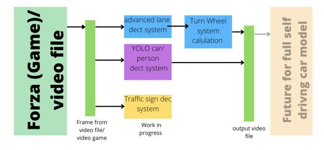
Simplified the 3 sections of a self driving car, my project is focused on the first part (feature extraction of the environment.
