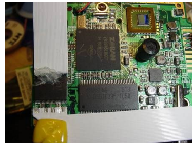
Hand soldered to exposed flex cables
