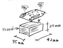
2 Put PCB and pedestal on the mesh. keep enough space between them. 十分に間隔を空けて配置
