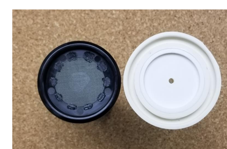
Internal of Filter Casing
