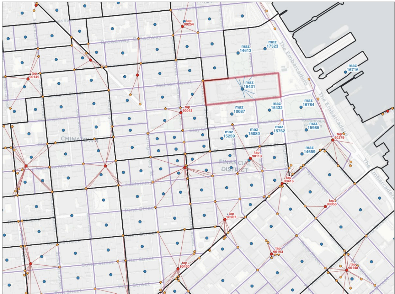
Figure 22: MAZ 15431 (red boundary), within TAZ 401 (dark black boundary), with MAZ centroids in blue, TAPs in red, and transit stops in orange
